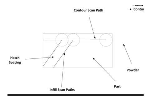
A compensated contour scan path that does not fuse material in the top right corner
